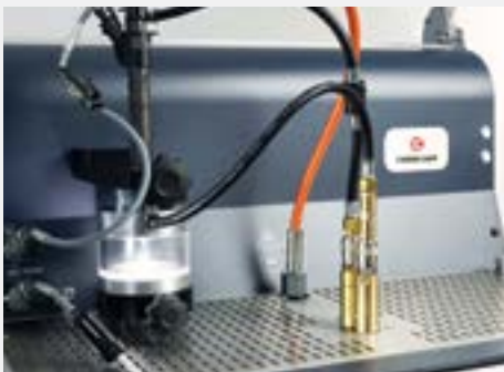
TESTING WITH ILLUMINATED SPRAY CHAMBER.
